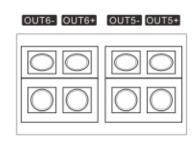
5CH+Signal output; 5CH-Signal output; 6CH+Signal output; 6CH-Signal output;
